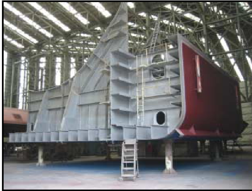
Figure 5. Mid-body bottom construction block.
